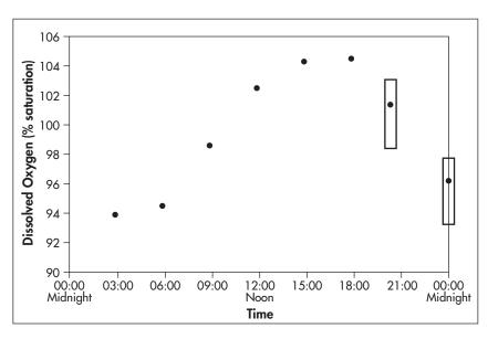
Changes in pond's dissolved oxygen saturation level over 24-hour period.
